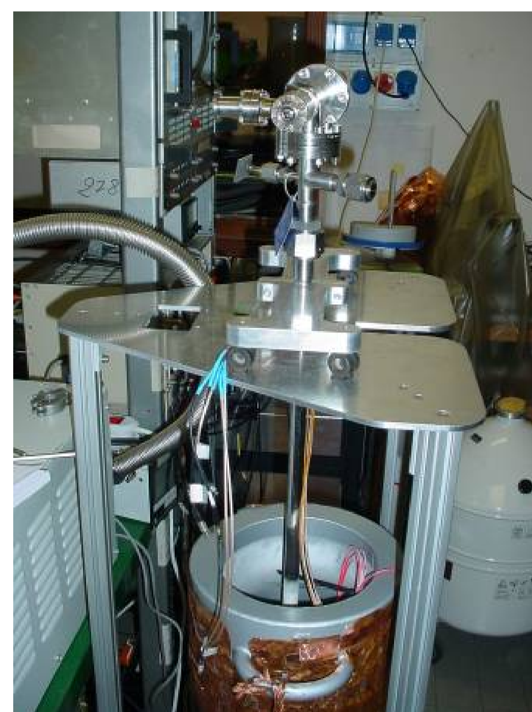
In order to simulate as much as possible the experimental set-up of the Gerda experiment, we used a specifically designed Dewar container filled up with liquid nitrogen to cool down an encapsulated p-type HPGe detector
