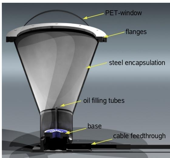
Figure 3. Sketch of the photomultiplier encapsulation
