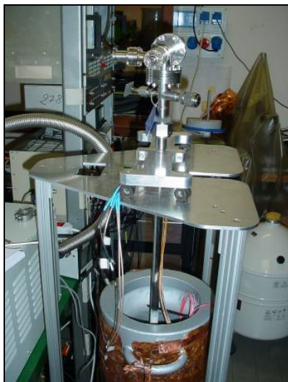
Fig. 2. The Dewar container and the associated mechanical holder allow relatively easy handling of the HPGe detector both inside and outside of liquid nitrogen.
