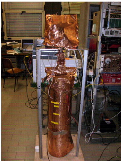
Fig. 1. Set-up of the energy resolution measurement test in Milan. The encapsulated germanium detector, Dewar container, mechanical holders and vacuum pump have been provided by the Gerda experiment.
