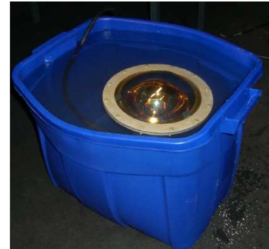
ETL 8" PM inside capsule with oil long term test in water
