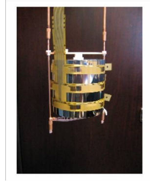
(c) segmented true coaxial n-type Ge detector for Phase II in low mass support and contact structures.
