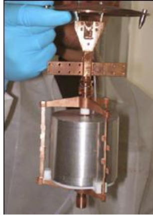
(b) p-type Ge detector for Phase I
