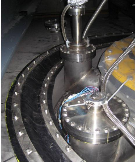
•EPDM rubber (ethylene propylene diene M-class rubber) is an elastomer which is characterized by wide range of applications. The E refers to Ethylene, P to Propylene, D to diene and M refers to its classification in ASTM standard D-1418. The "M" class includes rubbers having a saturated chain of the polymethylene type. The diene(s) currently used in the manufacture of EPDM rubbers are DCPD (dicyclopentadiene), ENB (ethylidene norbornene) and VNB (vinyl norbornene).
