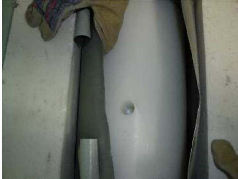
Figure 2 Detail of the hole made for source insertion. The remaining PE thickness is 1 cm
