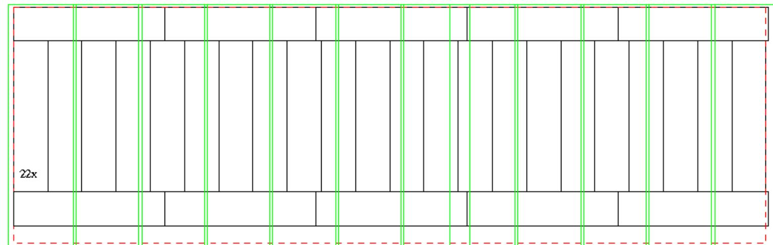
edges of VM2000 to be sealed with Scotch-Weld DP100 epoxy
