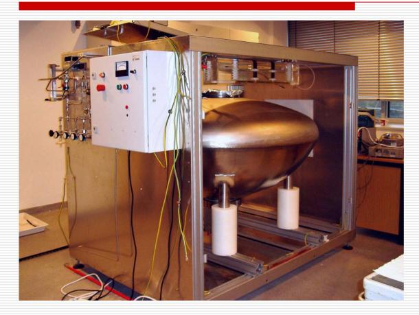
First calibration tests with larger PIN-diode (20×20 mm) have been performed
