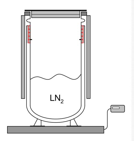
Additional insulation: foamed polystyrene and super insulation foil, improved lid
