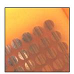
Cables laser welded to copper pins
