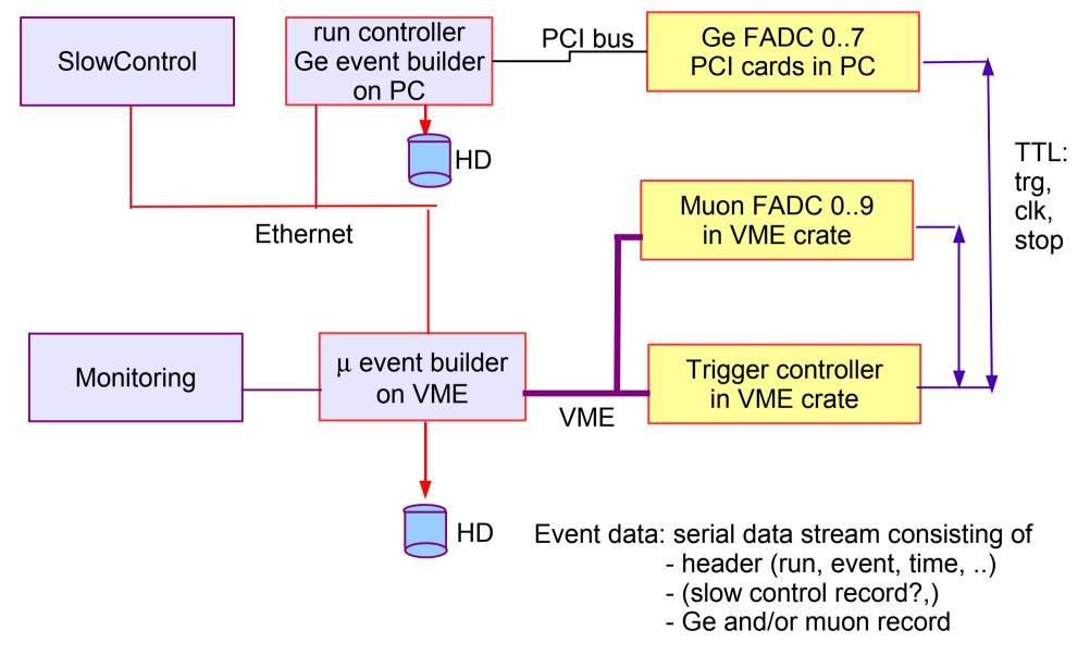
Ge and muon trigger independently a readout
