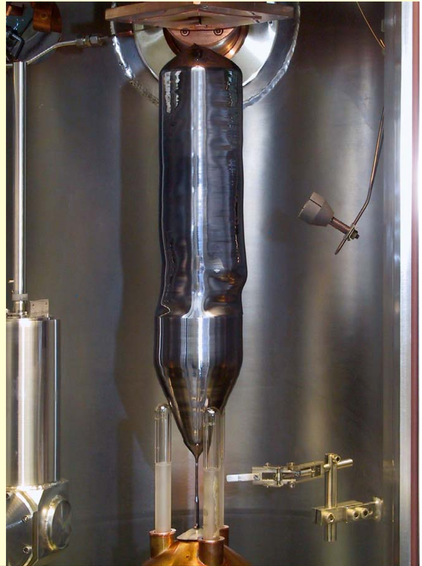
Dislocation-free Si FZ crystal with quadratic cross section
