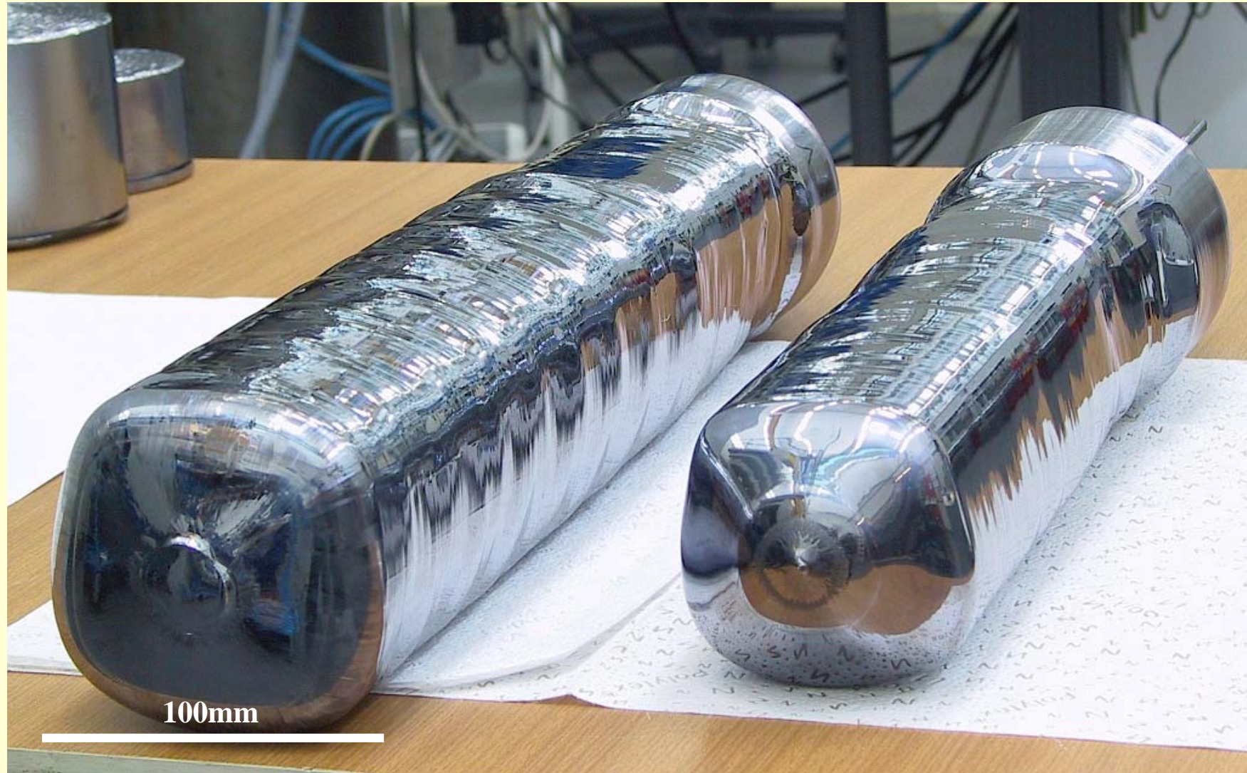
Quadratic FZ- silicon for high efficiency PV
