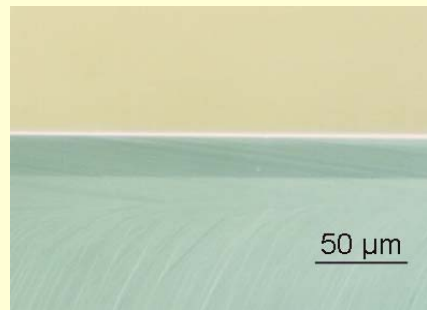
25 \mu\text{m} thick 4H-SiC-layer
