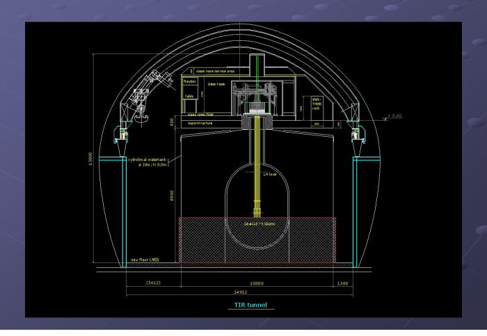
SS consists in 3 floors plus a platform for the lock system and its facilities (clean room and so on..)
