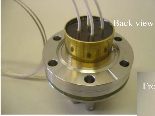
Other option: SHV Stycast insulated. Demonstrated to work at LNGS 1 month run+ multiple HV cycles in Ar atmosphere
