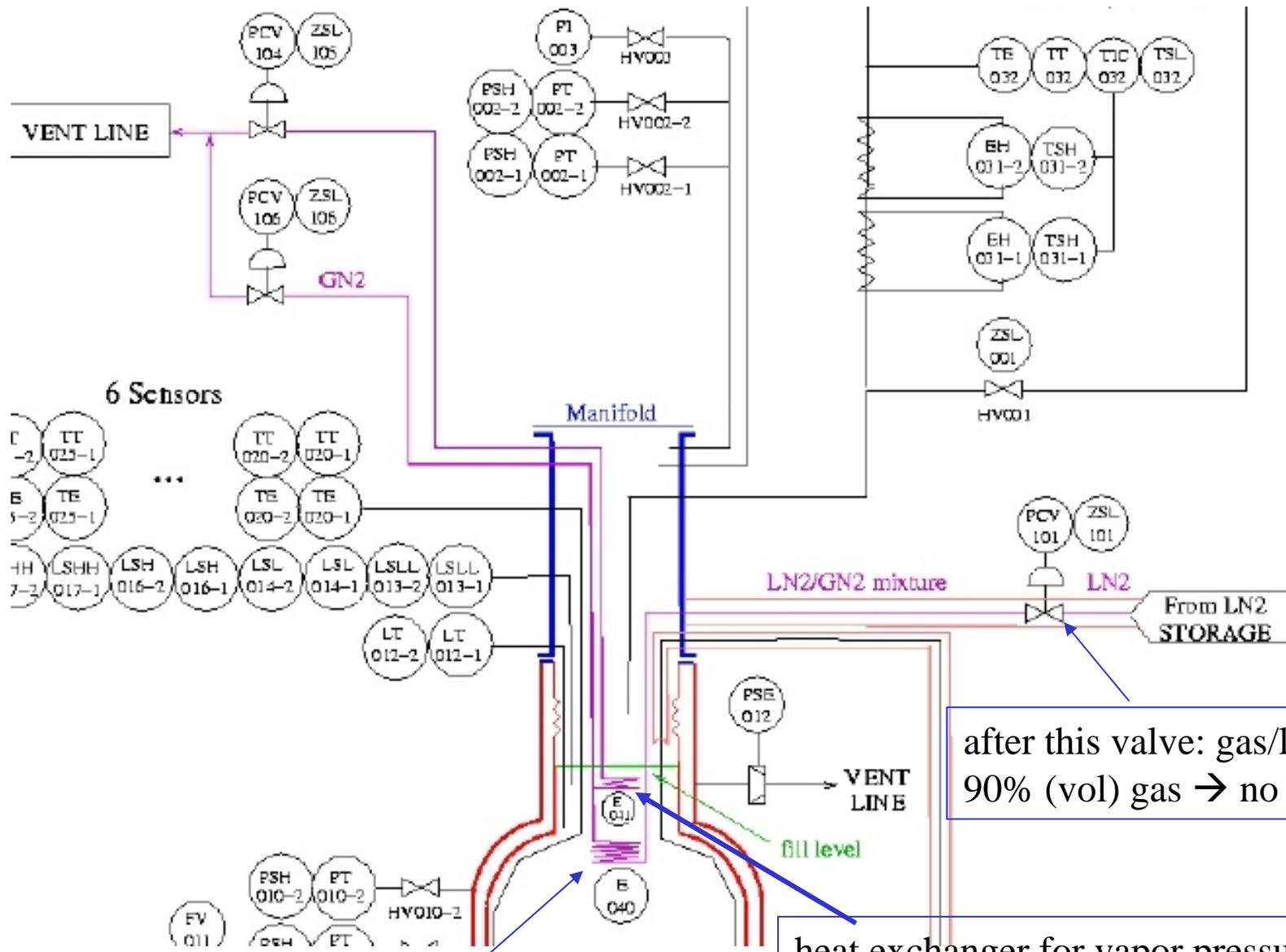
after this valve: gas/liquid mixture
