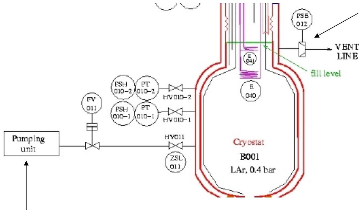
rupture disk: in case of a leak in the inner container
