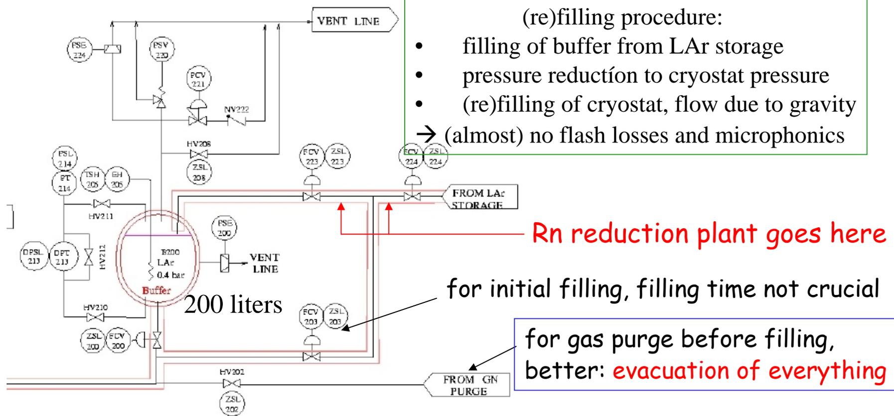
emptying: i) evaporation with heater: 2 weeks for 10 kW
