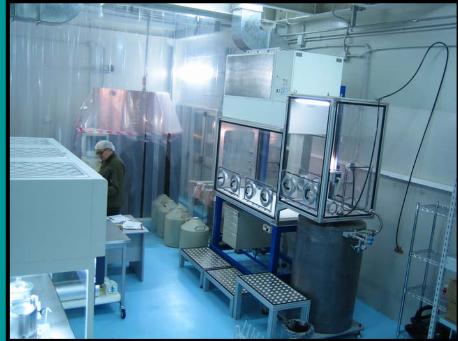
LARGE underground detector laboratory, LNGS, equipped with radon-free and normal clean bench.
