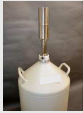
An environmental physics laboratory (top) where 3 germanium detectors are enclosed in their lead shields. An unshielded germanium detector (bottom) with the dewar for liquid nitrogen or liquid argon.
