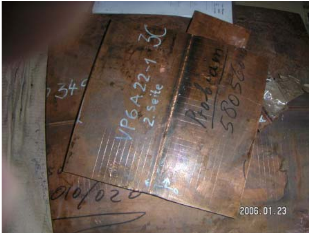
Pressing tests of EB welded 20 mm OFE copper sheets
