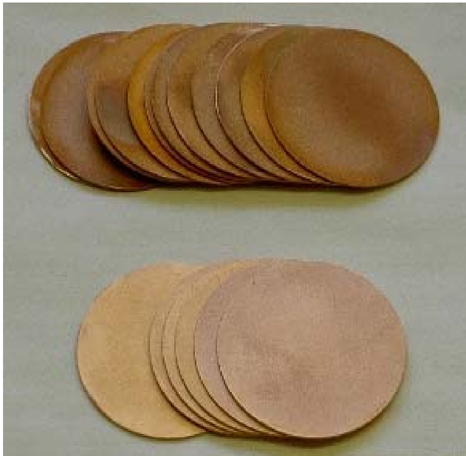
Discs before and after cleaning
