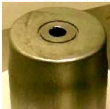
Photo of a refabricated RG3 (IGEX) HP 76 Ge crystal with the groove
