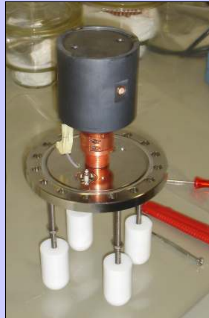
Crystal mounted on the cryostat flange.
