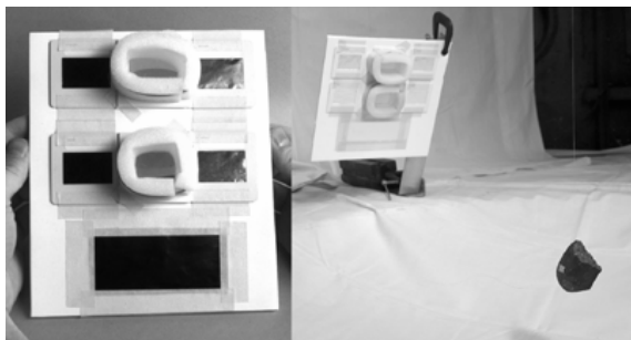
Figure 1. Passive particle detectors used in AVGR impact experiments to capture and measure the properties of dust-size debris. (Left) Detail showing the arrangement of foils and aerogel in a typical detector layout. ~7-, 13-, and 51- \mu\text{m} thick foils are set along the top, middle, and bottom rows, respectively, with blocks of aerogel set in foam holders between the foils. (Right) Typical deployment of a detector near a meteorite target within the AVGR impact chamber.
