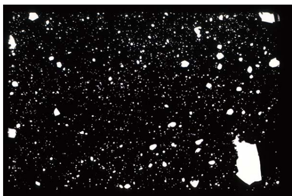
Figure 2. Slide scanner image of a 7- \mu\text{m} thick foil from detector 3 of AVGR shot 011015 (a 248-gm sample of
