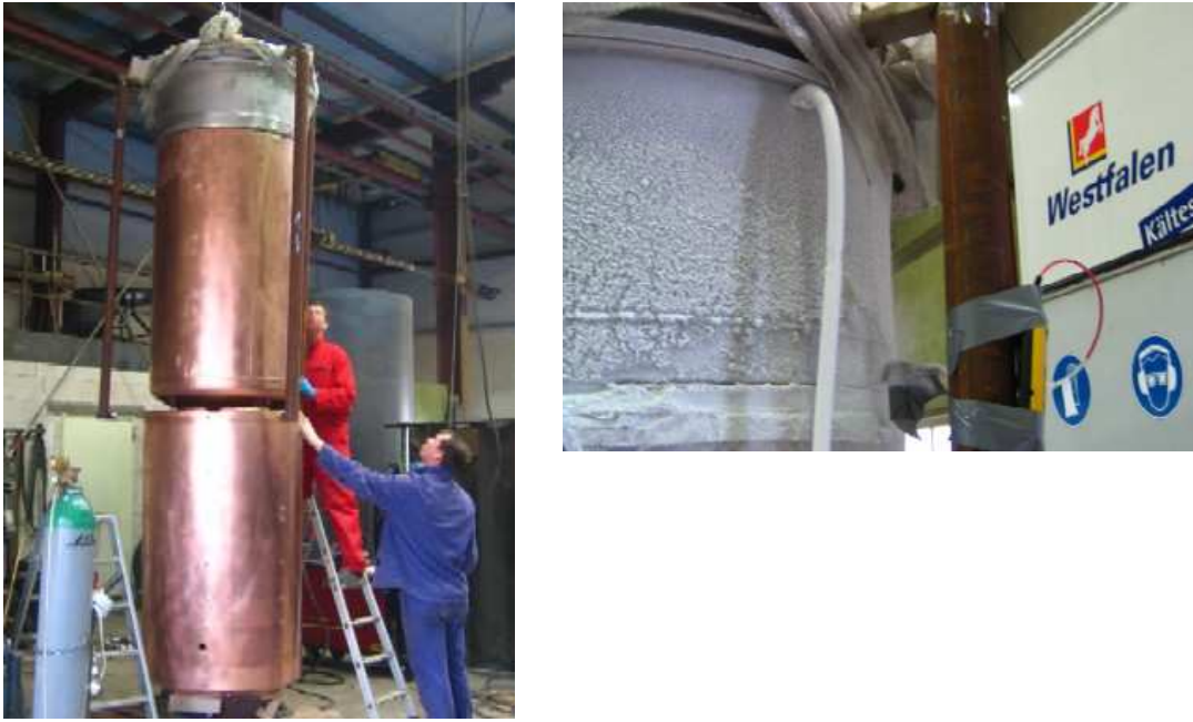
Figure 2: Left: Mounting of the thermal shield of the LARGe cryostat. Right: first cool-down of the integrated heat-exchanger after completion of the welding to the inner vessel and thermal shield.
