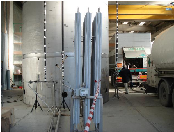
Figure 9: Set up for the evaporation test at SIMIC (left), and the measured evaporation rate during the settling time of the cryostat after being completely filled with liquid nitrogen.
