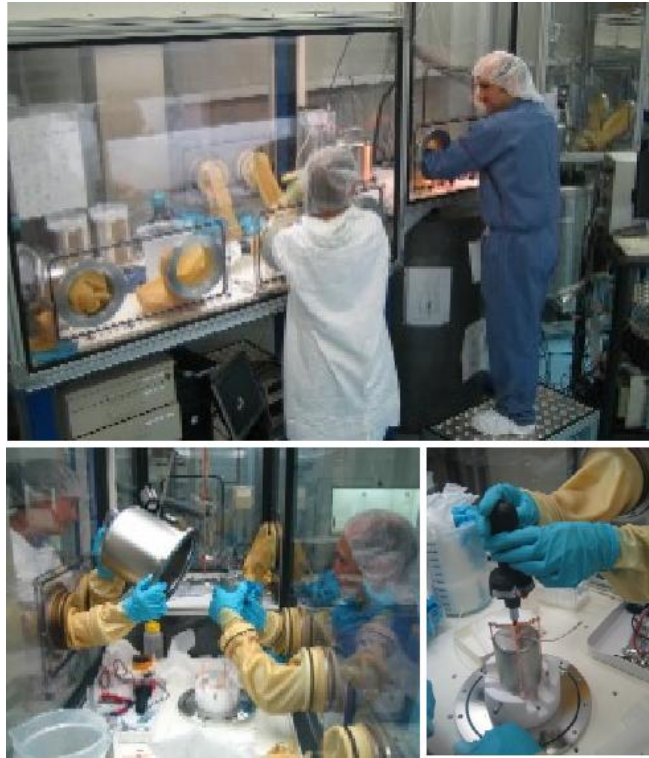
Figure 9: Top: Radon reduced glove-box/clean bench with nitrogen atmosphere and integrated liquid argon cryostat for mounting and testing the final phase I detector assemblies. Bottom left: Removal of an enriched crystal from its vacuum transportation and storage container. Bottom right: Adjustment of the torque of the high-voltage contact.
