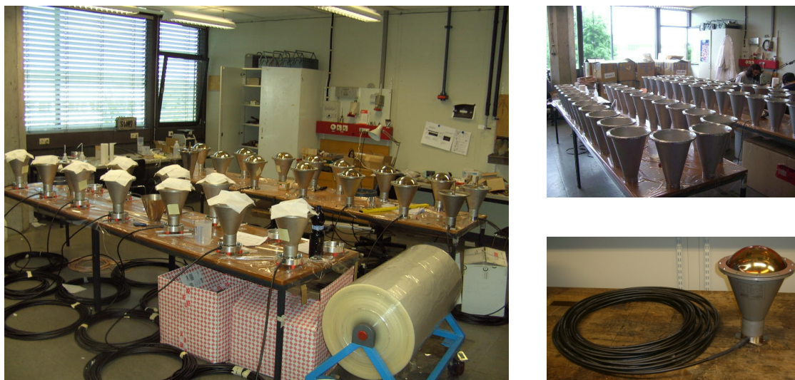
Figure 8: Left: During the production of the encapsulations of the PMTs at Tübingen. Right top: The array of capsules during cleaning. Right bottom: The encapsulated PMT ready for testing an packing.
